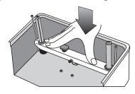
2. Before installing covers, please press "pushing bar" all the way down to the bottom, you will hear "click" then "pushing bar" will be held there.
